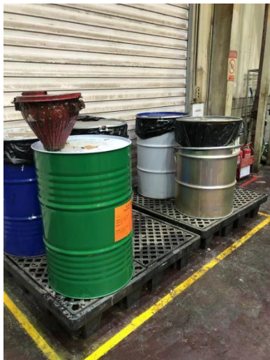
车间危废暂存区及托盘
